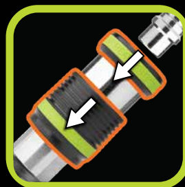
Pull sleeve down to shut off air flow and pull top collar down to disengage plug under zero pressure
