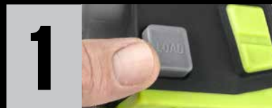
1 Press to release barrel
